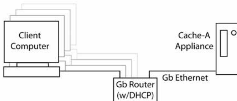
Archive Appliance Network Connection
